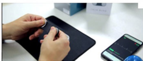
Figure 1. A single-channel mobile cardiograph is used to take an ECG from the fingers, followed by signal transmission via a smartphone to a center for spectral analysis
